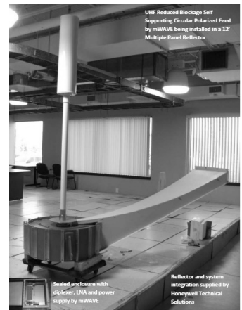
Feed Being Assembled In a 3.8m Reflector
